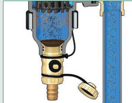
The collected debris can be discharge from the DIRTMAGPRO whilst the system is in operation by removing the ring and central magnets, opening the blow down valve and flushing through the debris.
